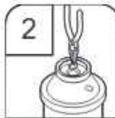
2. Use needle-nose pliers to remove plug.
