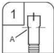
1. Fit rubber end (A) of drain hose to waste tee and cut if needed.
