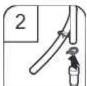
2. Attach drain hose to air gap with large drain hose clamp (provided). Use pliers to squeeze clamp open and move into position. If the drain hose was cut, use a 1½" to 2" (38 mm to 50 mm) screw-type clamp (not provided).
