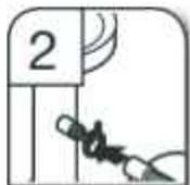
2. Attach rubber end of drain hose to waste tee with a large drain hose clamp (provided). Use pliers to squeeze clamp open and move into position. If the drain hose was cut, use a 1½" to 2" (38 mm to 50 mm) screw-type clamp (not provided).
