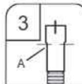
3. Connect rubber end (A) of drain hose to air gap and cut if needed.
