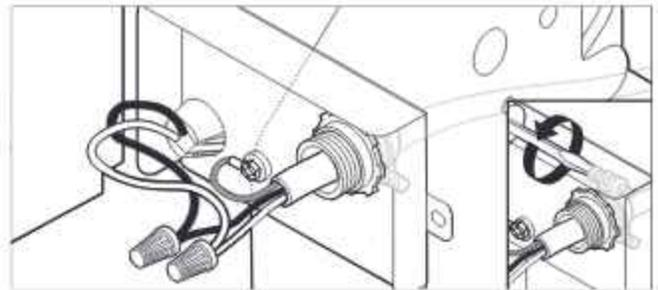
Tighten strain relief screws to secure cable.
