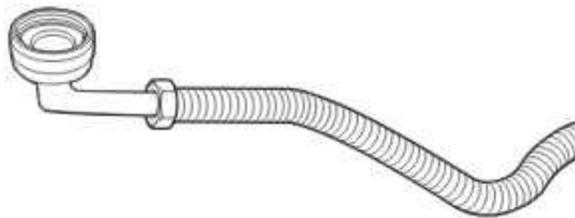
Get 3/8" (9.5 mm) compression x 3/4" (19 mm) hose fitting with 90° elbow. See the "Tools and Parts" section at the front of the guide for part details and order. Connect the 3/8" (9.5 mm) compression fitting of the 90° elbow fitting to the water supply line. Attach so the 3/4" (19 mm) connection is facing upward as shown above.
