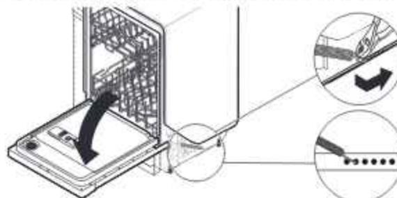
If the door falls open, increase the spring tension by moving the spring end toward the back of the dishwasher.
