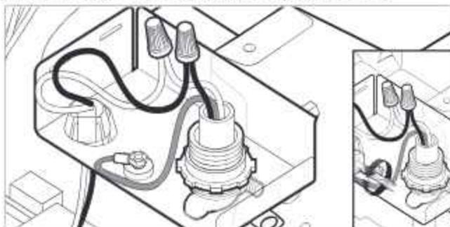
Tighten strain relief screws to secure cord.
