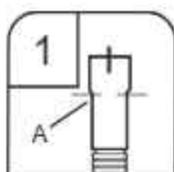
1. Connect rubber end (A) of drain hose to air gap and cut if needed.
