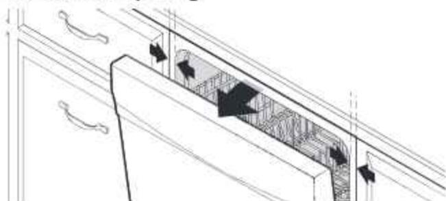
Open door and check that space between dishwasher cabinet opening and tub is equal on both sides. If spacing is not equal, loosen bracket screws and shift tub. Tighten bracket screws.
