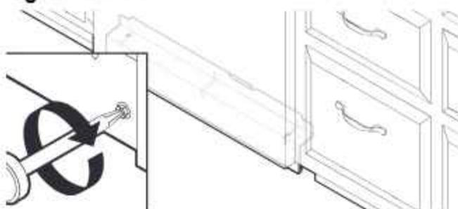
Tighten access panel screws.
