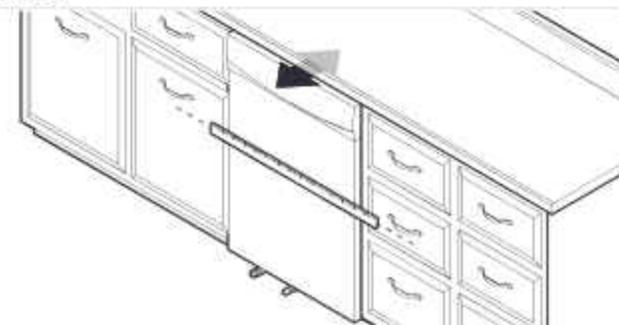
Align front of dishwasher door panel with front of cabinet doors. You may need to adjust alignment to be even with your cabinets.
