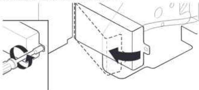
Using a 1/4" hex-head socket, nut driver, or Torx® T20® screwdriver, remove terminal box cover. Retain for later use.
