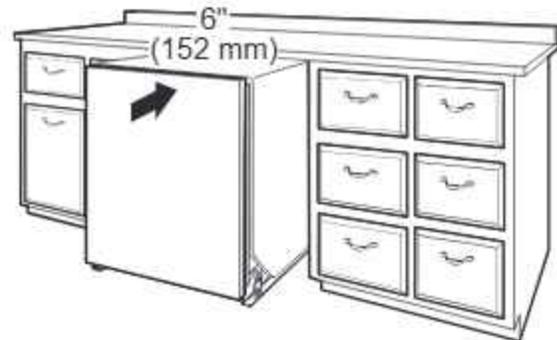
**NOTE:** Leave unit about 6" (152 mm) out from cabinet in order to install anchor brackets and adjust door tension if needed.
