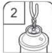
2. Use needle-nose pliers to remove plug.
