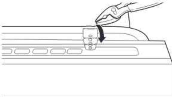
Using pliers, bend/twist tab to lock the brackets in place.
