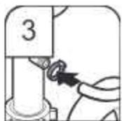
3. Use a rubber hose (not provided) with screw-type clamps (not provided) to connect from waste tee to air gap.
