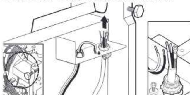
Route cord so that it does not touch dishwasher motor or lower part of dishwasher tub. Pull cord through strain relief in terminal box.
