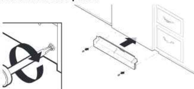
Place the panel against dishwasher legs. Using a Phillips screwdriver or 1/4" nut driver, reinstall the screws through the holes in the access panel.
