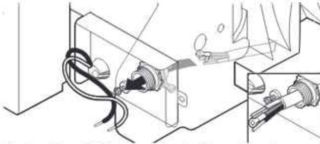
Route cable so that it does not touch dishwasher motor or lower part of dishwasher tub. Pull cable through UL-listed/CSA-approved strain relief in terminal box. Strain relief is not supplied with the dishwasher. Owner must purchase a 7/8" (22 mm) screw-in type strain relief.
