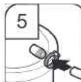
5. Use a rubber hose (not provided) with screw-type clamps (not provided) to connect from air gap to disposer inlet.
