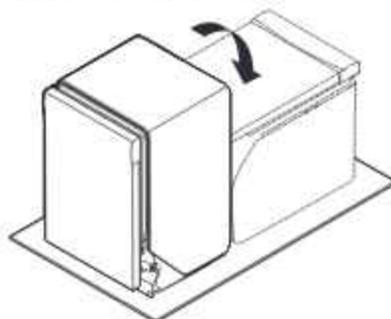
**Helpful Tip:** Place cardboard under dishwasher until installed in cabinet opening to avoid damaging floor covering.
