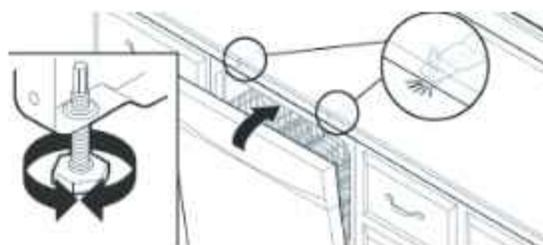
**IMPORTANT:** Check that top of door does not contact screws, brackets, or countertop. If it does, adjust leveling legs or use the side attachment option.
