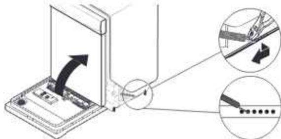
If the door closes too quickly, decrease the spring tension by moving the spring end toward the front of the dishwasher.
