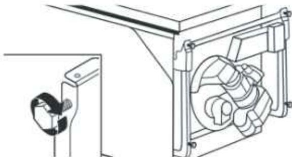
Refer to the "Dishwasher Height Adjustment Chart" for height of leveling legs needed for your cabinet opening.
