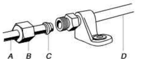
A. Line to ice maker B. Compression nut
