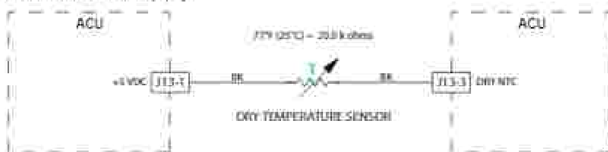
Figure 2 - Dry Temperature Sensor (NTC) Wire Diagram
