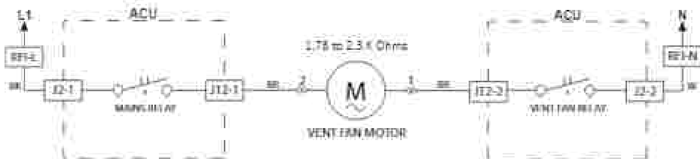
Figure 3 - Vent Fan Motor Strip Circuit
