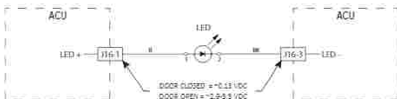
Figure 2 - Drum Light Drive Circuit
