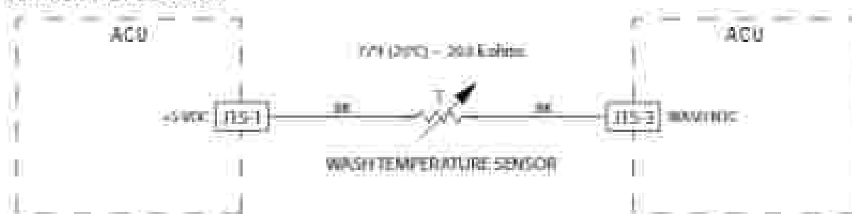
Figure 2 - Wash Temperature Sensor Wire Circuit
