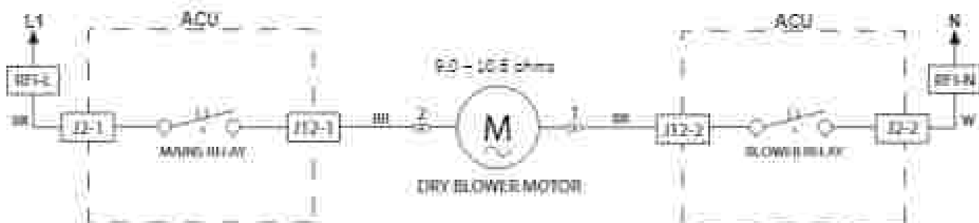
Figure 2 • Dry Blower Motor Wire Circuit
