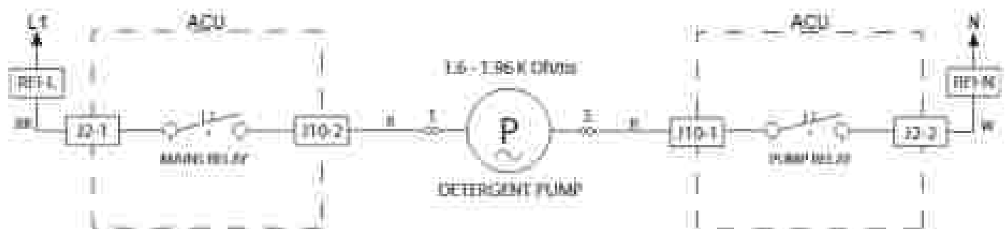
Figure 2 - Detergent Dosing Pump Wire Circuit
