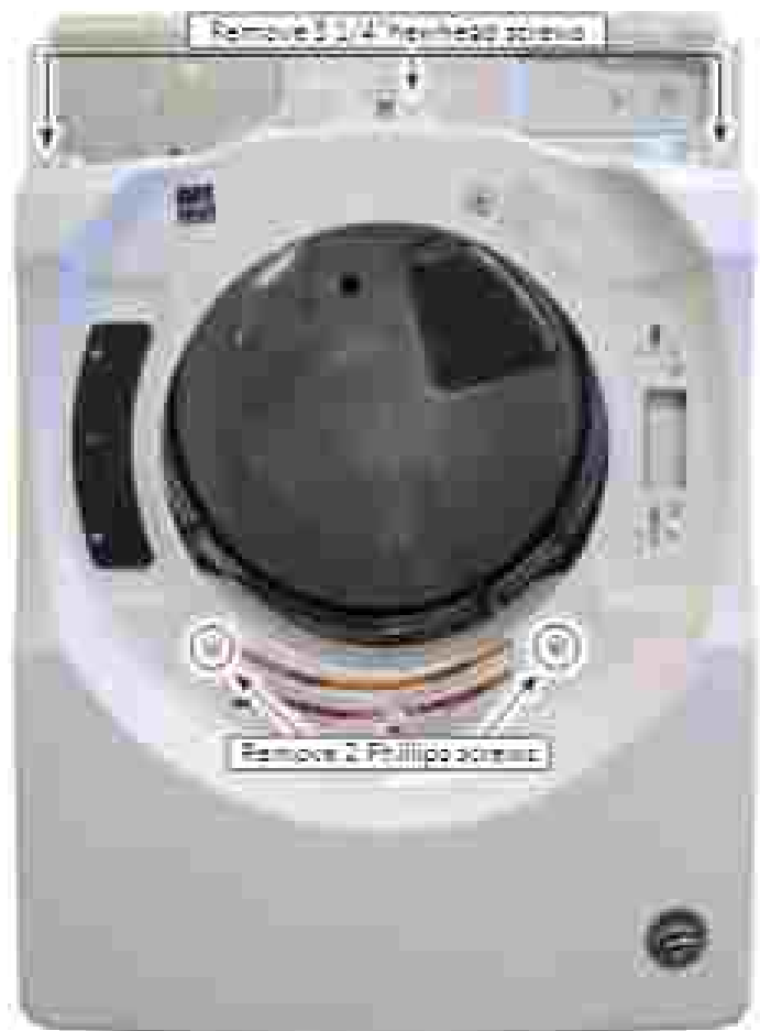
Figure 3 - Remove remaining screws on front panel.
