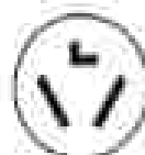
3-wire receptacle (10-30R)
