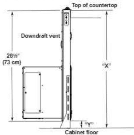
5. Attach the support legs to the side of the vent box with four 4 x 8 mm screws in each support leg. Adjust to dimension "Y" from the bottom of the vent box to the bottom of the support legs. Tighten screws.
