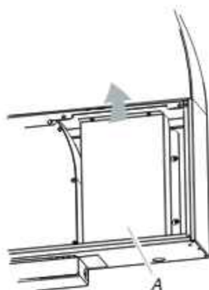
A. Terminal box cover
