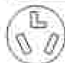
3-wire receptacle (10-30R)
