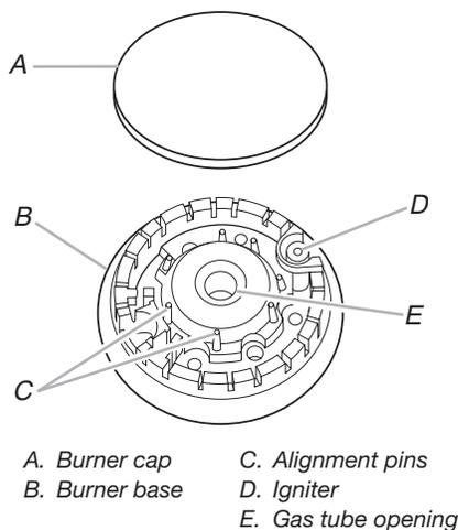
**Gas tube opening:** Gas must flow freely throughout the gas tube opening for the burner to light properly. Keep this area free of soil and do not allow spills, food, cleaning agents or any other material to enter the gas tube opening. Keep spillovers out of the gas tube by always using a burner cap.
