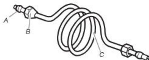
A. Compression sleeve B. Compression nut C. Copper or PEX tubing
