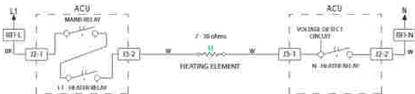
Figure 3 - Wash Heating Element Schematic Circuit
