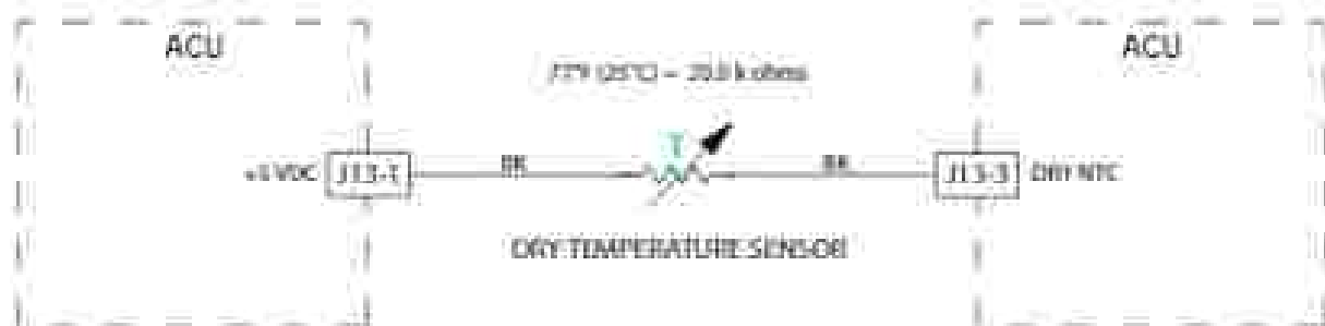
Figure 2 - Dry Temperature Sensor (NTC) Wire Diagram
