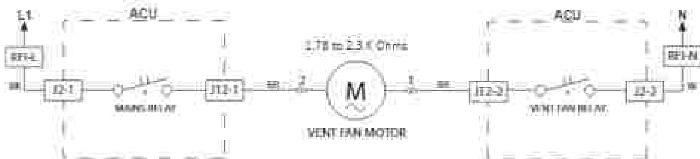
Figure 3 - Vent Fan Motor Strip Circuit
