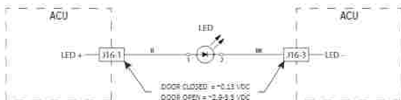
Figure 2 - Drum Light Error Circuit
