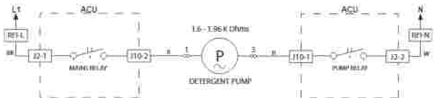
Figure 2 - Detergent Dosing Pump Wire Circuit
