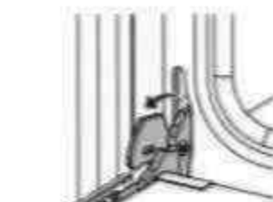
Oven door hinge lock in unlocked position
