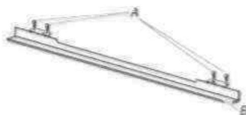
A. Philips head screws (4), only 2 screws for 27" (68.6 cm) size B. Deflector (1)
