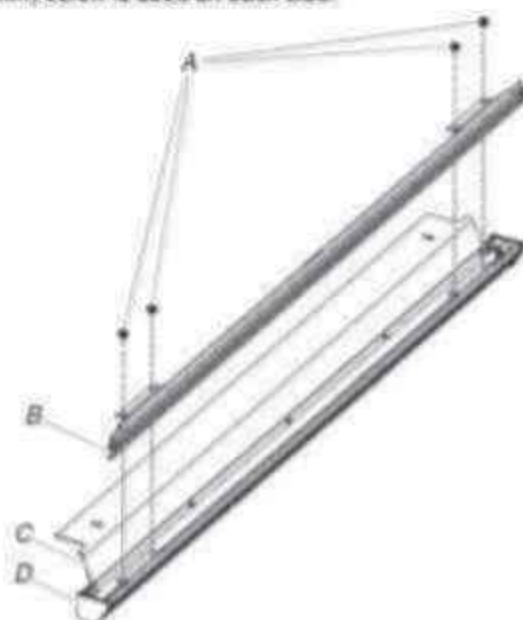
A. #8-18 x 1/4" (6.4 mm) screws B. Deflector C. Upper vent piece D. Lower vent piece
