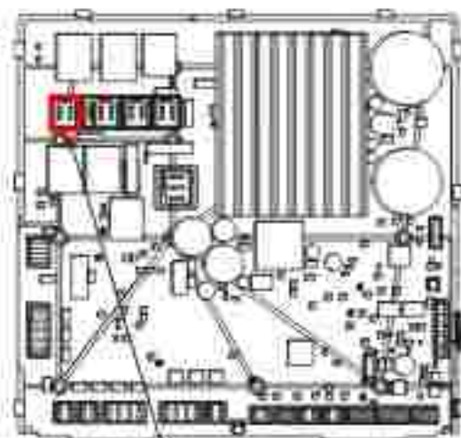
Figure 2 - Location of Dry Heater Connector on ACU
