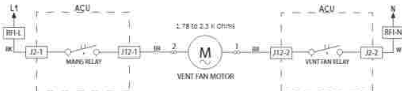
Figure 3 - Vent Fan Motor Strip Circuit
