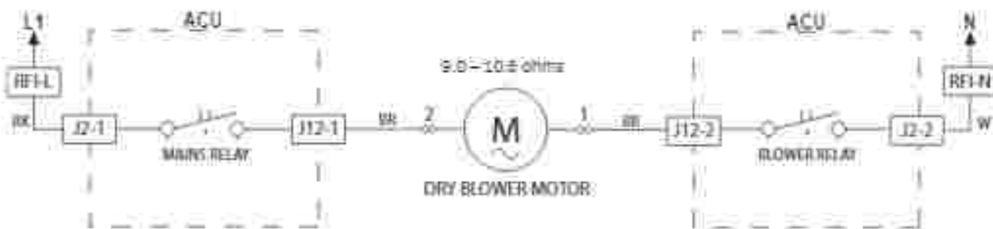
Figure 2 - Dry Blower Motor Strip Circuit
