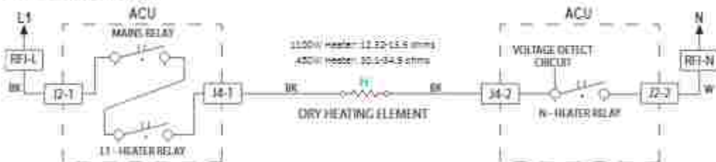
Figure 3 - Dry Heating Element Strip Circuit
