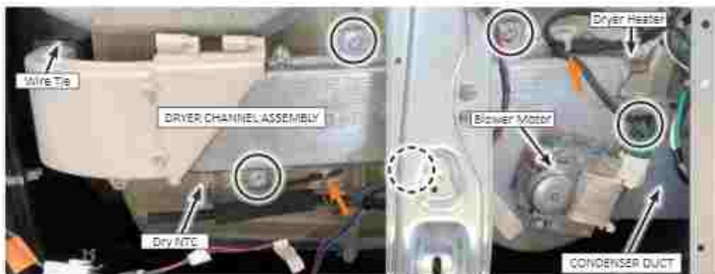
Figure 1 - Dryer Channel Assembly
