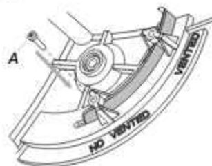
A. No Vented method screw
