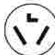
3-wire receptacle (10-30R)
