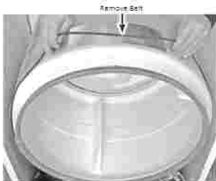
Figure 5 - Remove drum belt.
