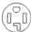
4-wire receptacle (14-30R)
