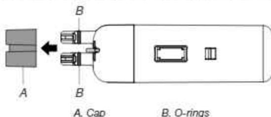
5. With the arrow pointing up, align the new filter with the filter housing and slide it into place. The filter cover door will automatically begin to close as the new filter is inserted.
