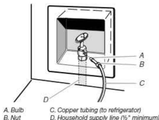
4. Now you are ready to connect the copper tubing to the shutoff valve. Use  $\frac{1}{4}$ " (6.35 mm) O.D. (outside diameter) soft copper tubing to connect the shutoff valve and the refrigerator.
