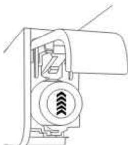
1. Locate the water filter in the top-right corner of the refrigerator compartment.
