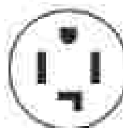
4-wire receptacle (14-30R)
