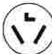
3-wire receptacle (10-30R)
