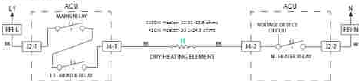
Figure 3 - Dry Heating Element Schematic Chart
