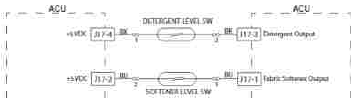
Figure 2—Bulk Dispense Level Sensing Schematic
