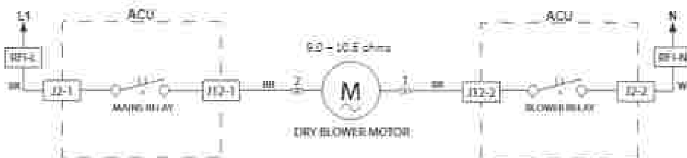
Figure 2 • Dry Blower Motor Schematic Circuit
