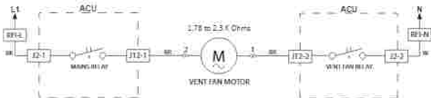
Figure 3 - Vent Fan Motor Strip Circuit
