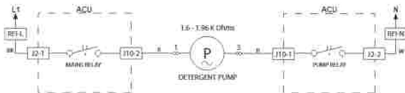
Figure 2 - Detergent Dosing Pump Wire Circuit
