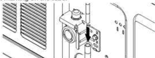
Inserting water line into guide
