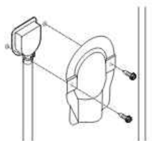
Water line cover
